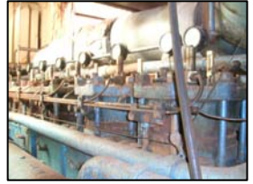
Jakobs hovedmaskine: B&W/ Alpha Diesel, 409-26VO
